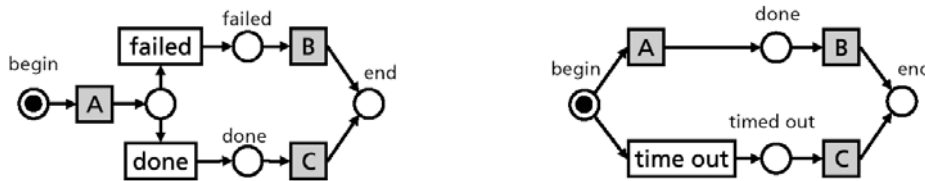
Fig. 8. Two examples of explicit, user-defined fault management. If A fails, B will be executed; if A completes successfully, C will be executed ( left ). If A does not complete after a specified time out, C will be executed. If A completes in time, B will be executed ( right )
