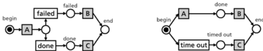
Fig 7: Two examples of explicit, user-defined fault management. Left side: If A fails, B will be executed; if A completes successfully, C will be executed. Right side: If A does not complete after a specified time out, C will be executed. If A completes in time, B will be executed.
